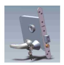
A Privacy Key Facility is also provided allowing a secondary privacy bolt to be locked or unlocked by a key operated rim cylinder lock on the outside and anti-ligature furniture on the inside. The Privacy bolt can be overridden by extending and then withdrawing the main bolt and a clutch mechanism ensures that staff remain in control. The cylinder is also master keyed to provide staff control of the privacy mechanism.
