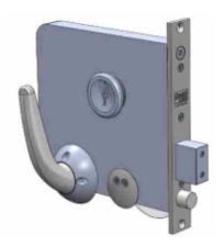
A privacy facility is also provided allowing a secondary privacy bolt to be locked or unlocked by anti-ligature furniture from the inside of the accommodation. The privacy bolt can be overridden by a key holder by extending and then withdrawing the main bolt. A clutch mechanism fitted to the internal furniture ensures that staff members always remain in control of the privacy bolt.
