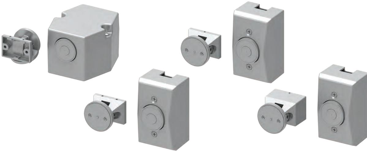
The Sentronic® SEM 7800 Series are heavy duty, electrically controlled door holding magnets. Magnets are fail safe and hold until the current is interrupted. A manual door closer is used to control and close the door. A choice of floor, recessed wall, or surface mounted wall magnets are available.
