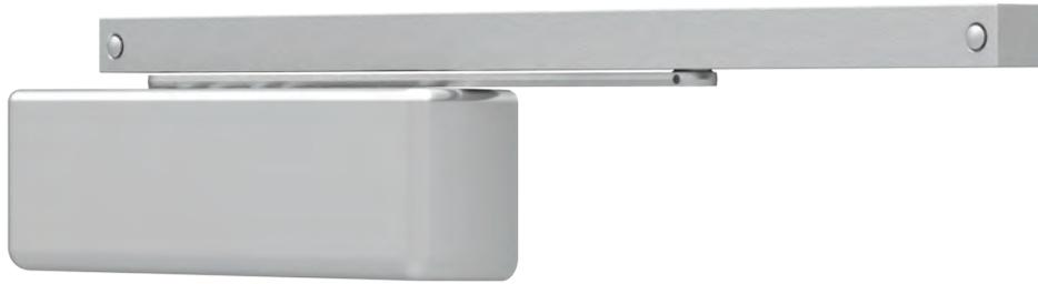
The 4040SE SENTRONIC<sup>®</sup> is a heavy duty, non-handed, nonsized closer/holder designed to provide single point hold-open for fire and smoke barrier doors. The door is held open until current interruption releases the holding mechanism and the door closes. Single lever (track) arm closer is specifically designed for interior doors. Choice of finishes, track functions, and installation accessories meet virtually all life safety requirements.
