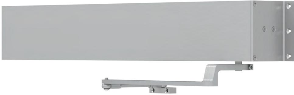
The 9540 SENIOR SWING by LCN is an ADA door operator that is a two-in-one swing door operator. SENIOR SWING operators when activated, opens doors automatically for wheelchair access, yet allows for manual operation for regular pedestrian traffic.
