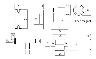
**Note:** Width of case increases from 19mm to 23 mm for 3579 series SCEC lock
