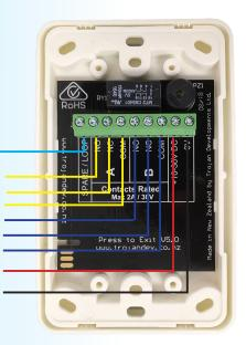
Spare / Loop terminal for other terminations Set "A" Contacts connect to the Request to Exit input on the Access Control door module. You might need an EOL resistor.
