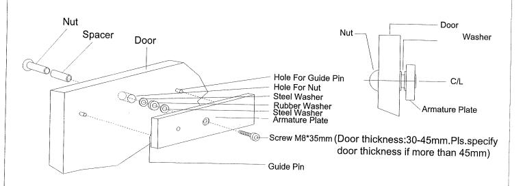
\*\*Important: Fix the armature plate not too tightly and make the rubber washer more flexible,in order to make the armature plate automatically adjust its proper position with the magnet.
