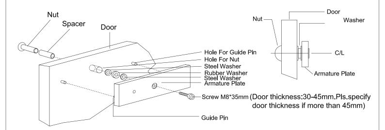
\*\*Important: Fix the armature plate not too tightly and make the rubber washer more flexible,in order to make the armature plate automatically adjust its proper position with the magnet.
