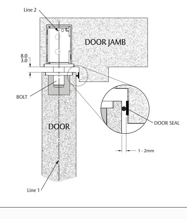
When determining the location of the strike and the lock, always ensure the door seal is not overcompressed against the door jamb.
