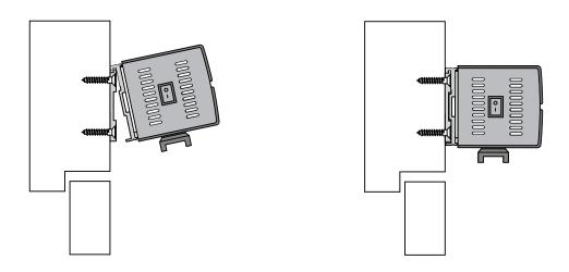
Hook the operation system on the finished base plate as shown, fix it with eight hexagon socket head screws.
