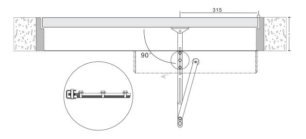
Loosen this three bolts and adjust the push arm length according to the door depth(L) until the angle between the push arm and door panel is  $90^\circ$ .
