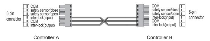
Note: Two doors share same sensor or same signal source, both doors may hold open, in this case, exchange two signal wires of the sensor which is connected with the same controller, it doesn't matter controller A or B.
